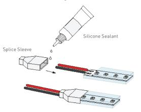
On the end that connects to power, use a sharp tool to peel back the silicone coating in order to expose the solder pads.
