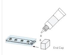
1. Seal any uncovered ends with an end cap. Use silicone sealant to ensure a waterproof fit.
